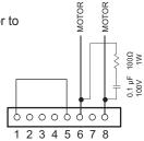
14. With power OFF, connect encoder to 8-pin connector as shown in diagram:
